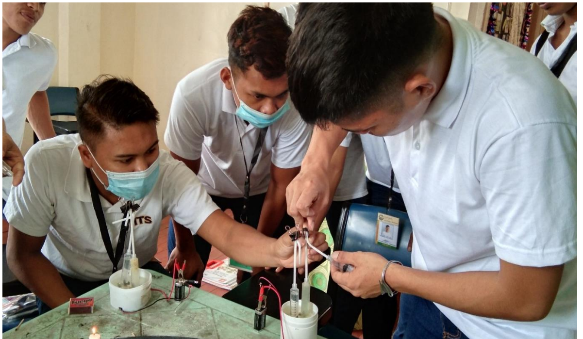
Grade 7 and 11 students setup an improvised electrolysis apparatus to breakdown water to hydrogen and oxygen gas.
